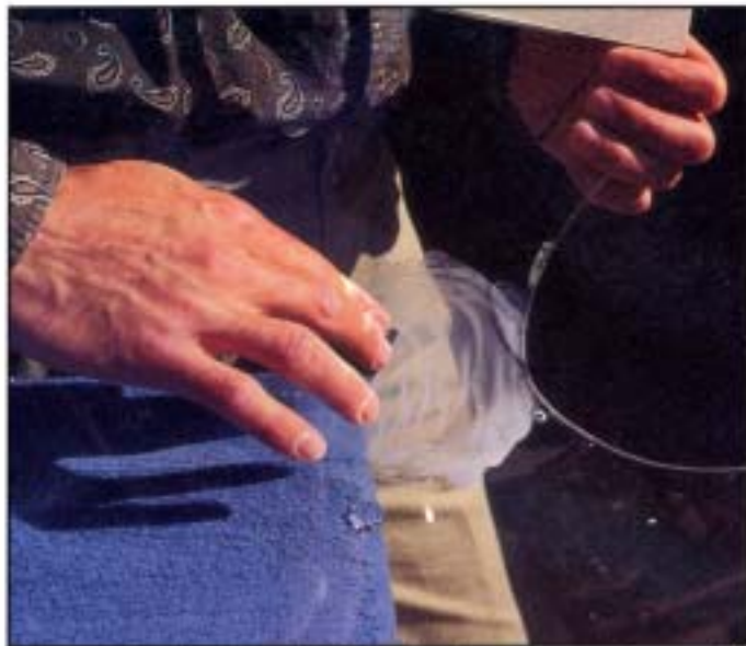
Wet sanding the area with 600 grit wet-or-dry sandpaper until the scratches cannot be felt with the fingernail.
