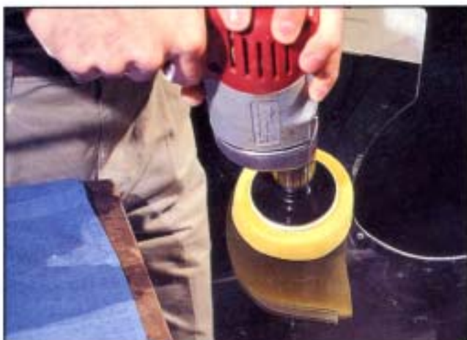
The coarser yellow pad goes to work with the drill turning medium slow and a small amount of pressure being applied. This is only for a few minutes.
