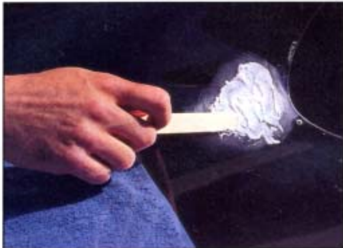
Applying the SO-1 Micro Cut compound.
