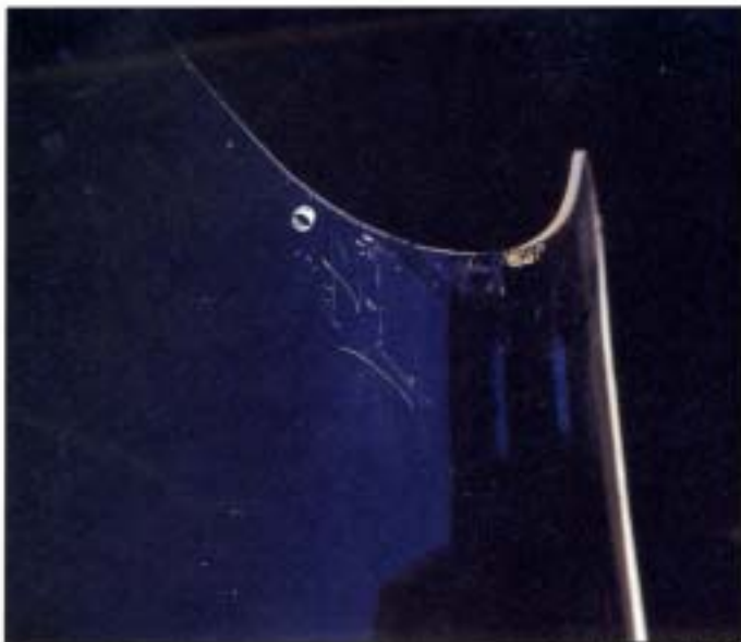
The problem: the series of scratches next to the drilled hole in the windshield.
