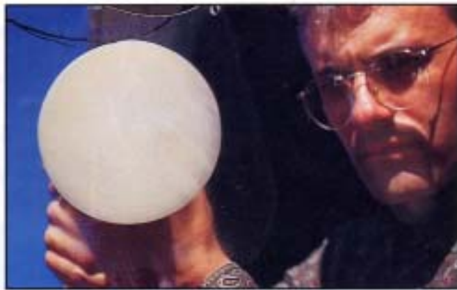
Steps 3 and 4 are done with the white VELCRO™ pad and SO-3 Micro Brite and SO-4 Micro Shine. Each brings the area closer to the original clear PLEXIGLAS.
