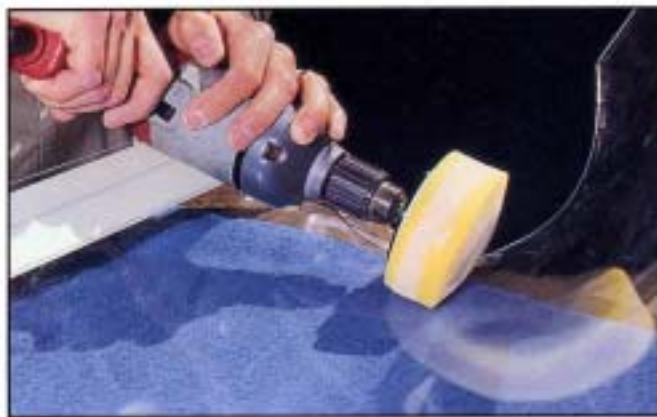
Step 2 shows an alternate way of using the edge of the pad to smooth out the PLEXIGLAS with SO-2 Micro Lite
